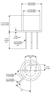
Bipolar PNP Device in a Hermetically sealed TO39 Metal Package.
